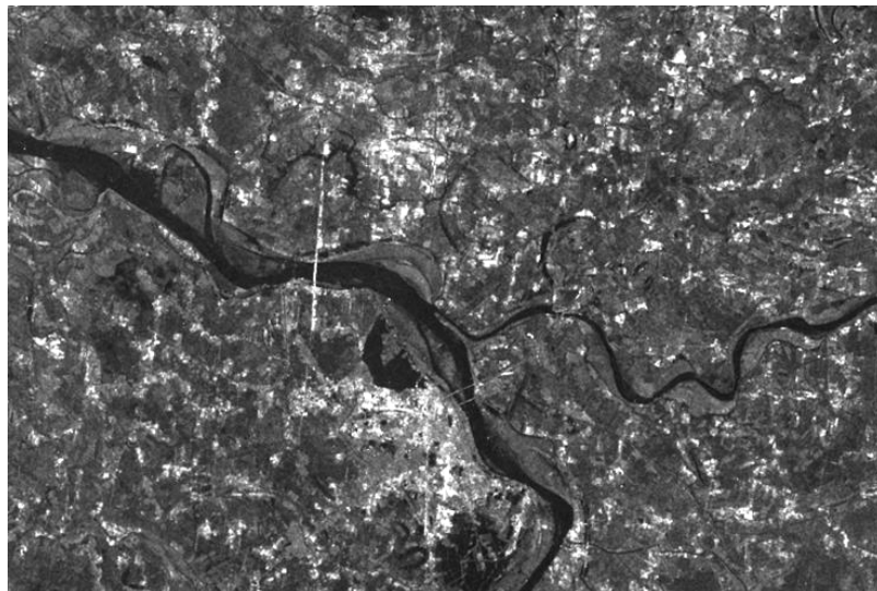
Figure 3.1: JERS-1/SAR image 30 m resolution after processing of GAMMA 3X3 FILTER and Orthogonal Geometric Correction
