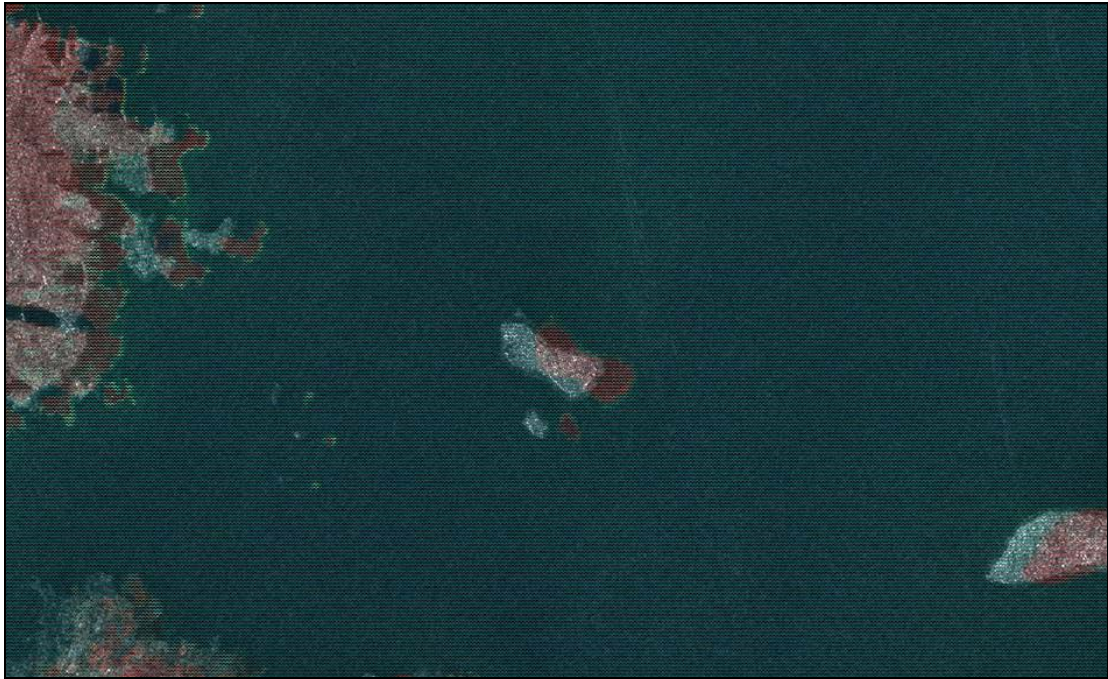
Figure 2.9: Different position of objects between ALOS/AVNIR-2 and ALOS/PALSAR data (Red layer is ALOS/AVNIR-2 image. White layer is ALOS/PALSAR image)
